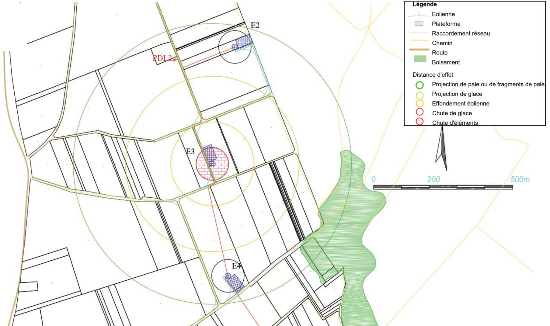
FIGURE 51 : CARTOGRAPHIE DE SYNTHESE DES RISQUES – EOLIENNE E3
