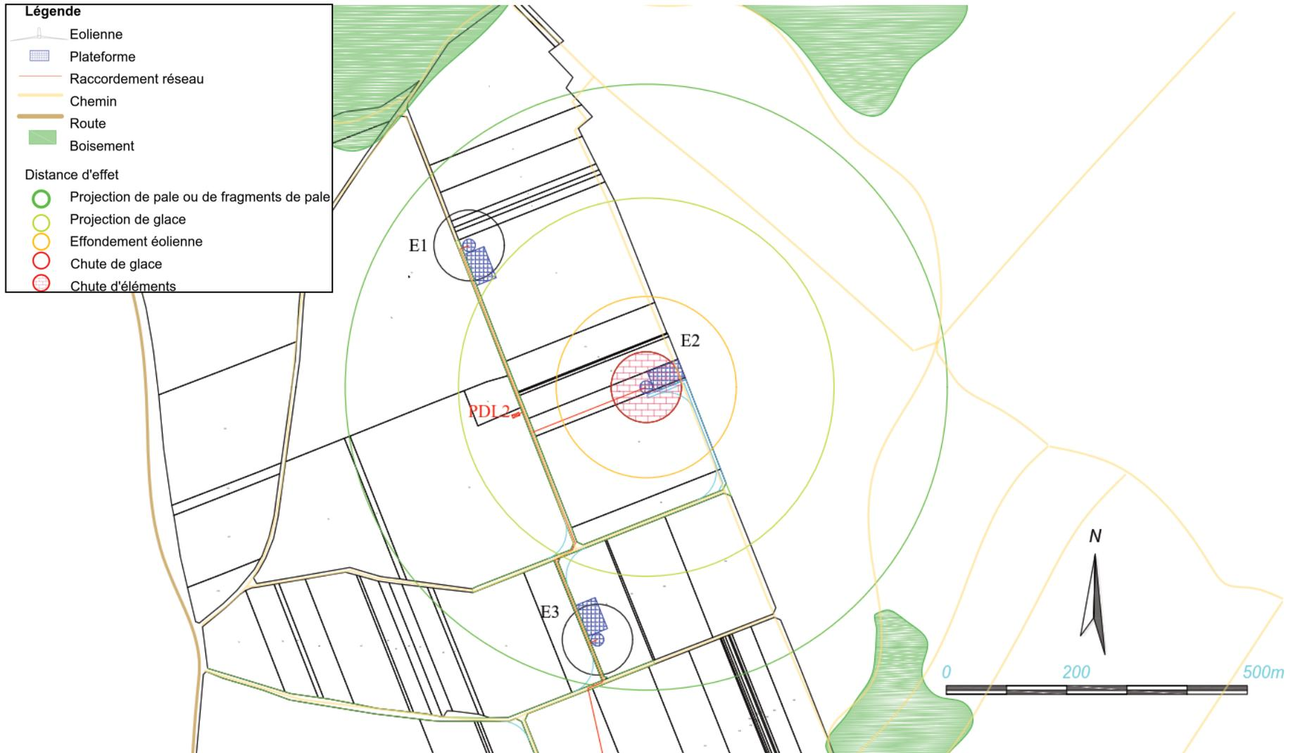
**FIGURE 50 : CARTOGRAPHIE DE SYNTHESE DES RISQUES – EOLIENNE E2**
