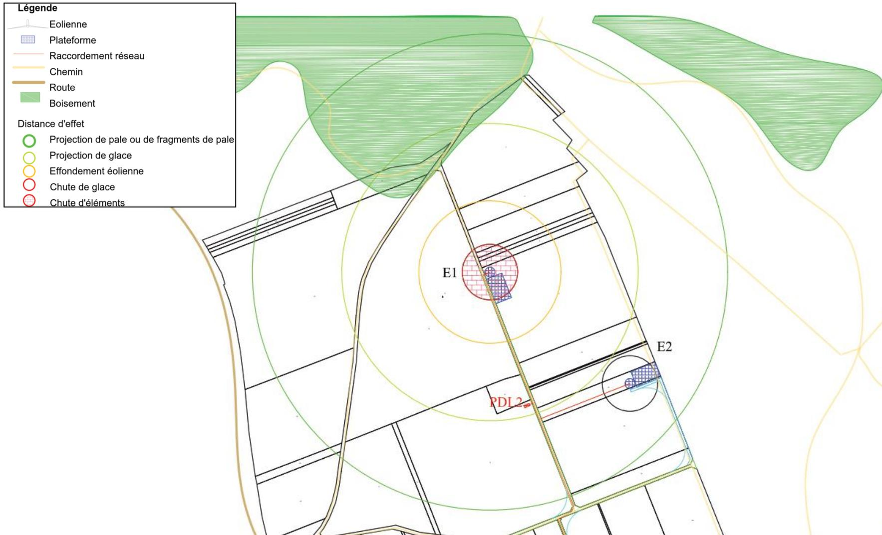
**FIGURE 49 : CARTOGRAPHIE DE SYNTHESE DES RISQUES – EOLIENNE E1**
